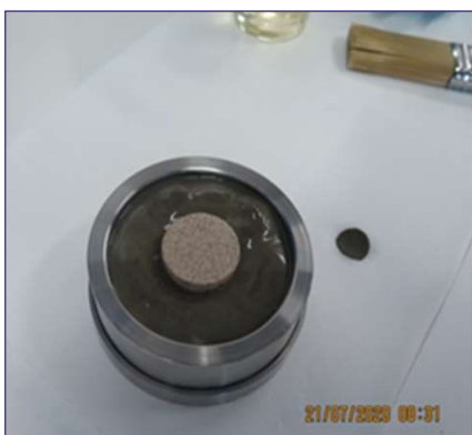
Push-out mould with sandstone and cement slurry for shear bond tests at IFPEN
